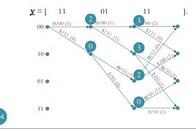
Each **circled number** at a node is the running (cumulative) path metric, obtained by summing branch metrics (distance) up to that node. Here, it is simply the cumulative distance.
