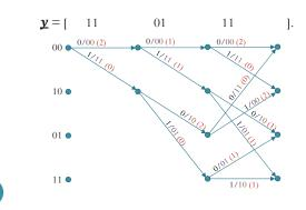
The number in parentheses on each branch is the branch metric, obtained by counting the differences between the encoded bits and the corresponding bits in  $\boldsymbol{y}$ .
